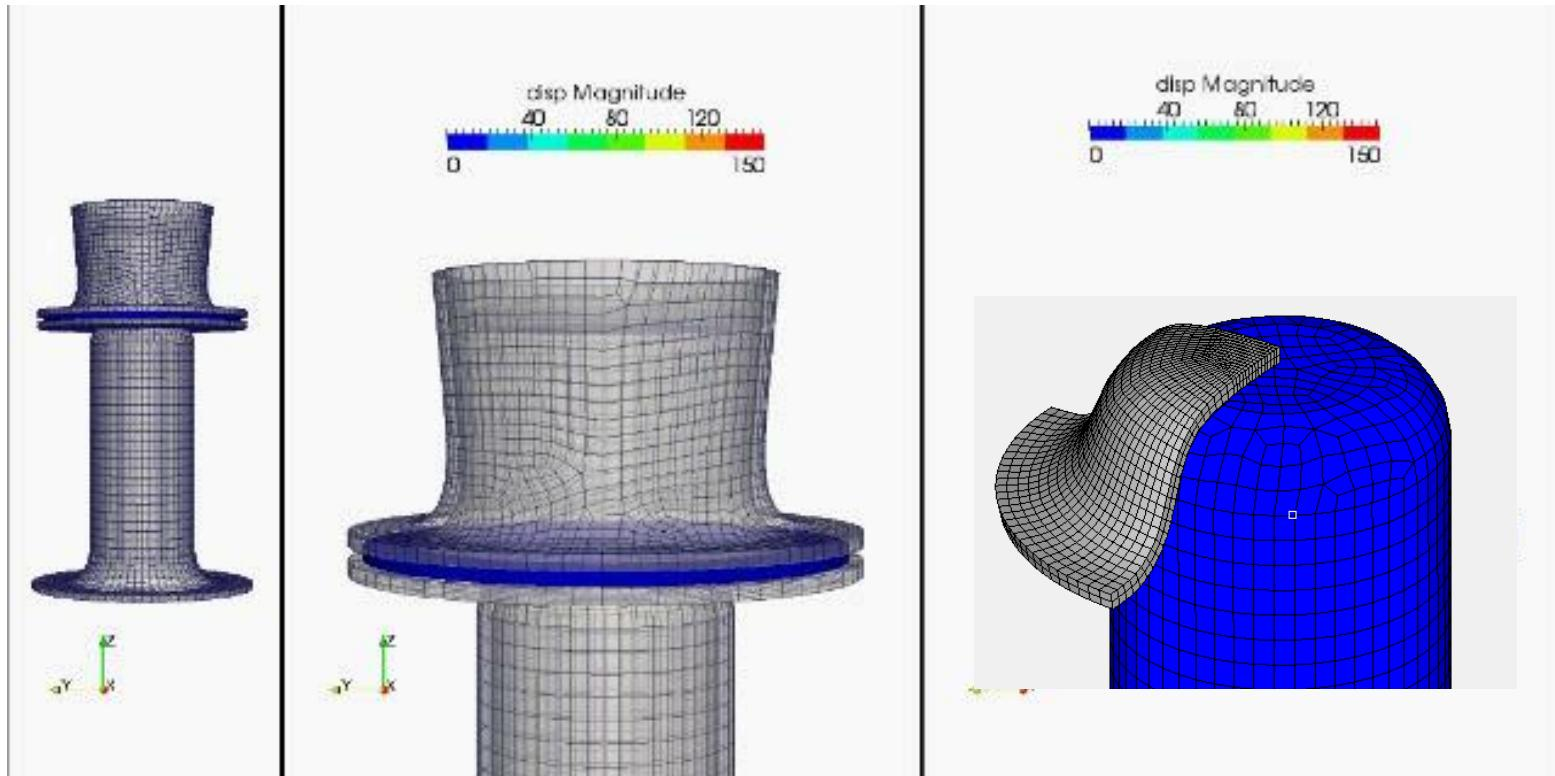
A punch is plugged into a blank, which is placed between a die and a blank holder. The blank is formed into a cylinder shape as the punch is plugged.
